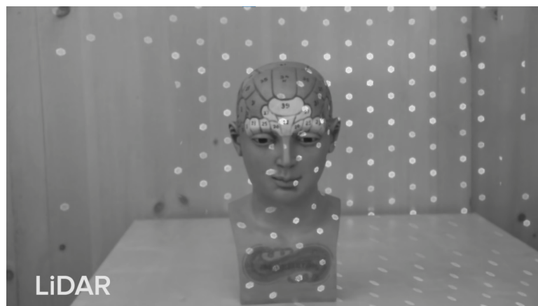
Figure 4.3: IR camera displaying the point density of the iPad LiDAR sensor [33]
