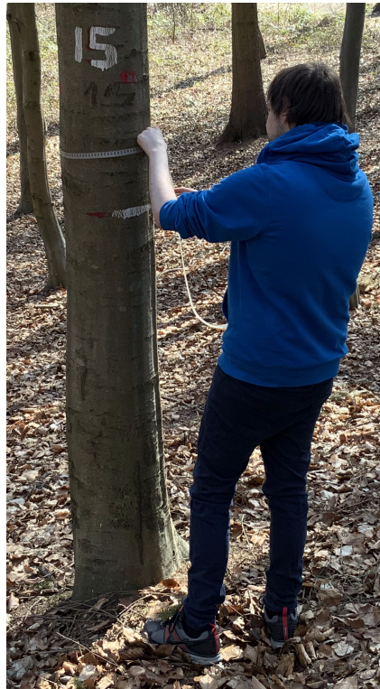
Figure 3.1: In-field DBH measurement with a measuring tape
