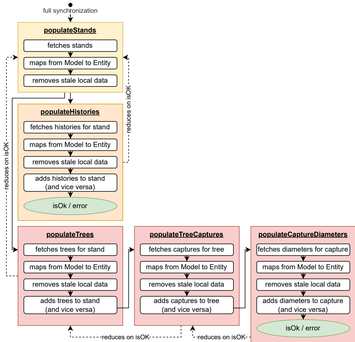
Figure 6.15: High-level view of a full local database synchronization
