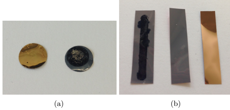
Figure 2.3: (a) Picture of both sides of the round samples, (right) showing the cathode layer facing upwards, and (right) showing the deposited nanowires as the black spot. The metallic dots are nanowires which have overfilled the template. (b) Picture of rectangle shaped samples. To the left is a template after deposition of nanowires (black area). In the middle is a template before deposition and to the right is a template with the cathode layer facing upwards.
