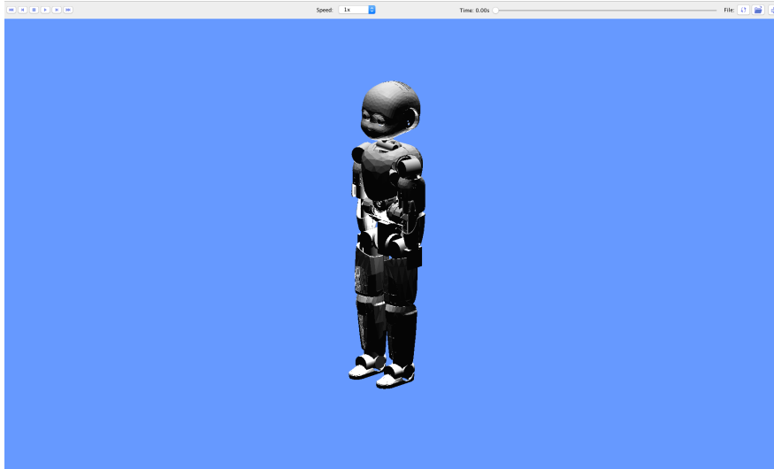
Figure A.15: Screenshot of the MBSysPad Animation 3D Model for the generated iCub MBS file
