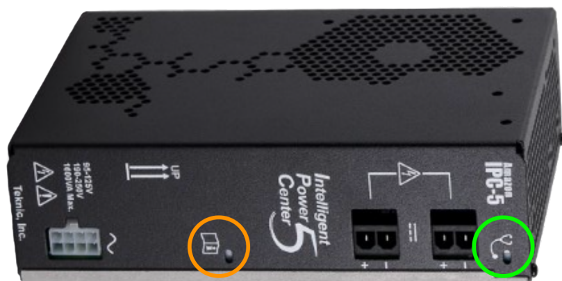
Figure F.3: If the bulb circled in orange is lit, indicating an orange light, an overvoltage has occurred. If the bulb circled in green is lit, indicating a green light, the system is functioning correctly.
