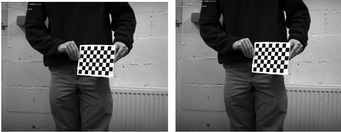
Figure 5.6: Camera calibrated image example, original (left) undistorted (right).
