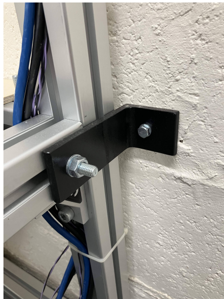
(c) Attachment device used to reduce vibration.
