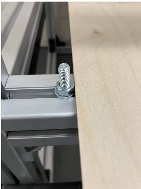
(a) One of the screws allowing the plank to glide in the same position every time.
