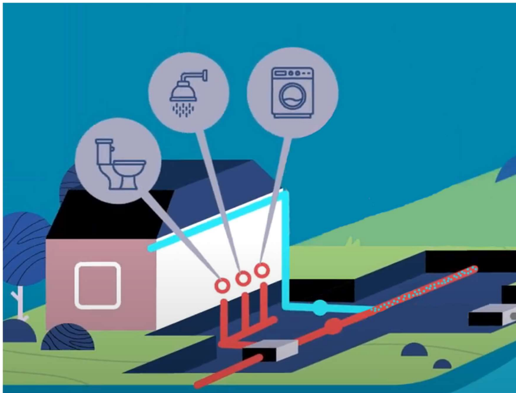
Figure 2-3: Illustration d'un mauvais raccordement [21].
