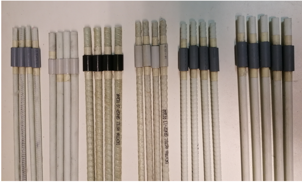
Figure 3.6: FRPs with their anti-adhesive region made with a PVC tube.
