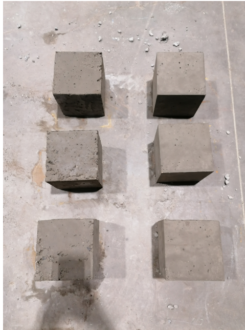
Figure 3.2: Standard cubes for concrete quality tests
