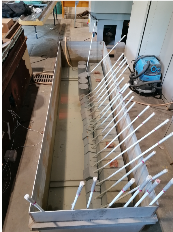
Figure 3.8: Storage of the samples in a tank filled with tempered water.
