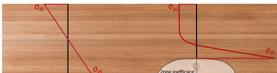
FIGURE 1.4 – Redistribution des contraintes de flexion
