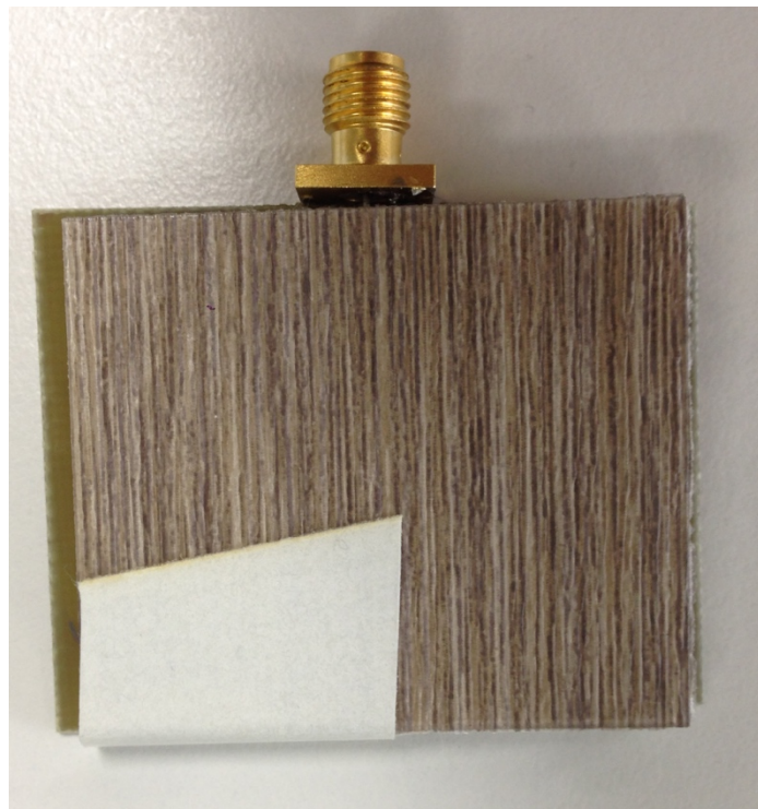
Figure 38 - Up side picture of a unique patch combined with an upper layer
