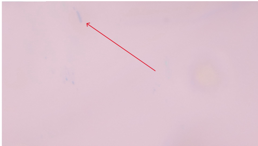
Fig. 3.13.: Optical image of leftover piece of CrSBr that remained on the stamp after first transfer.
