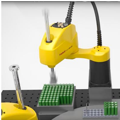
(a) SCARA robot on a production line
