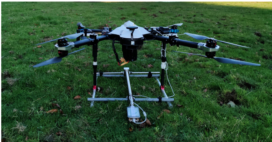
Figure 4.6 – Drone-borne GPR set up used for field measurements including the antenna linked to a VNA, GPS device, microcomputer and its power bank
