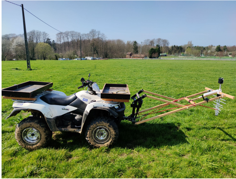
Figure 4.7 – All-terrain vehicle holding the GPR system, including the antenna linked to a VNA, GPS device, microcomputer and its power bank.
