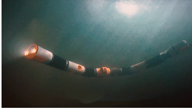
Figure 1.4: Eelume is an example of industrial applications of eel-like robotics: this subsea robot is used in inspections, maintenance and repairs for oil and gas installations. Images courtesy of [5].
