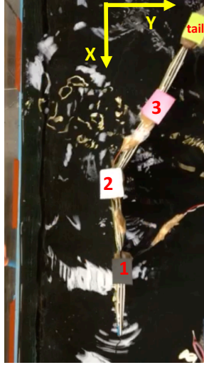
Figure 2.5: Experimental setup: the N = 4 links eel-like robot swimming forward in the LEFT hall pool. Image acquired by a camera (Iphone 6) placed atop the scene.
