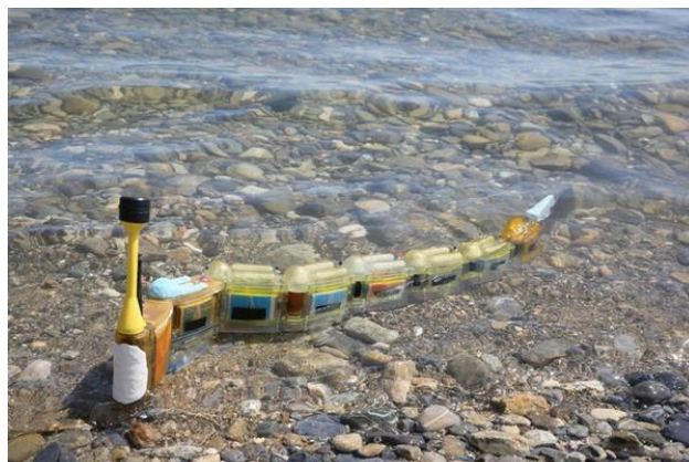
Figure 1.3: Envirobot is capable of detecting pollutants present in water in real time. Images courtesy of [4].
