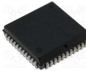
Figure 5 — Example of chip carrier [20]
