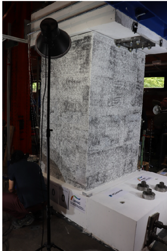
Fig. 4.11.: Speckle pattern on the East flange and Web of UW1 at LS0 (i.e., prior to loading)
