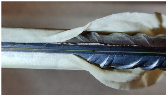
Fig. 4.12.: Close-up of the 12 mm reinforcing bar with optical fiber attached
