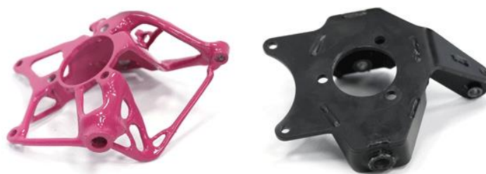
Figure 2-7 Optimized part (left) and original part (right) [14]
