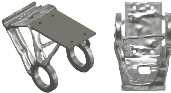
Figure 4-6 Die casting in the lateral direction (=direction of the ring axis)
