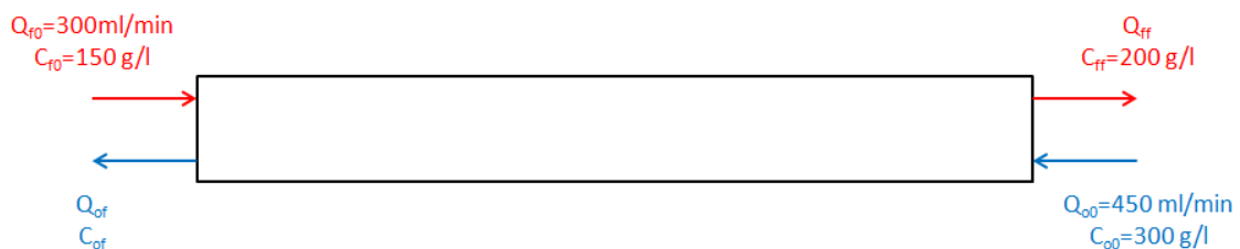
Figure 5.13: Schema of one module. Q is the flow, C the concentration. Index f refers to the feed, o to the osmotic, 0 means it is the initial value, f the final one.
