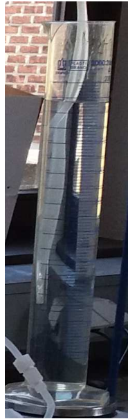
Figure 4.4: Disposition of the tubes in the feed column. The upper tube brings the feed solution towards the membrane. The lower one brings back the solution with potentially crystals.
