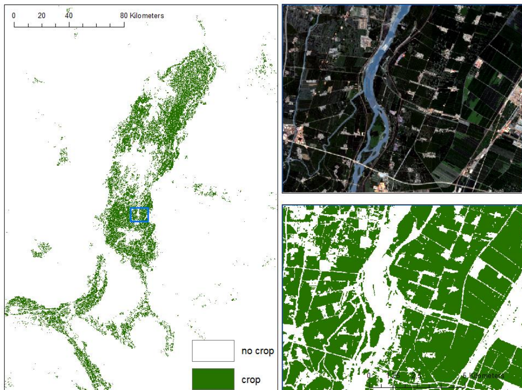
Figure 16: Mask A. Binary crop land mask generated in Sen2-Agri, with in situ reference data. The whole study area (left), a zoomed in section (extent in blue on the main map) as a Sentinel-2 composite of July (top right) and as the cropland mask (bottom right).
