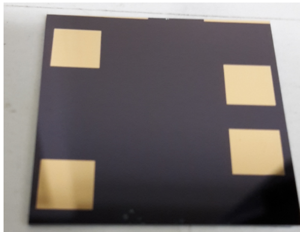
Figure 36: Sample before bismuth deposition. 24mm*24mm Si (100) with 90 nm thick SiO 2 and gold contacts (30nm) deposited on top of a 5 nm Ti layer (for adherence on the substrate).
