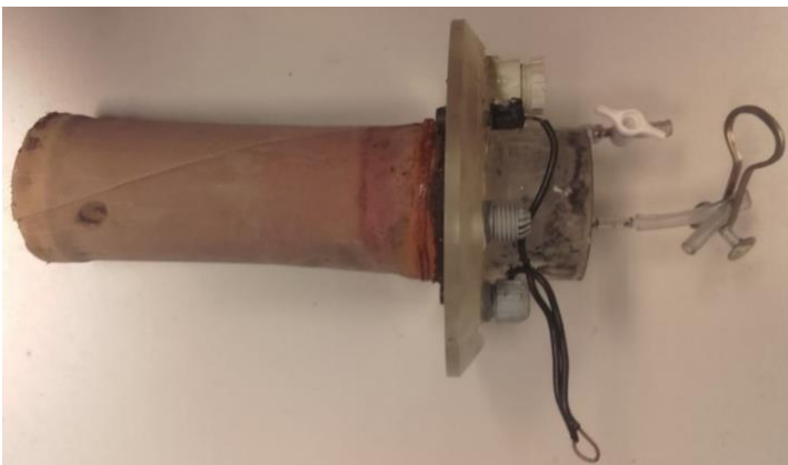
Figure 3-6 : EF membrane sealed to the cap of the reactor. The black wire are the cathode connexions, the white screw is the pH probe hole, the two grey screw sampling tubes holes.
