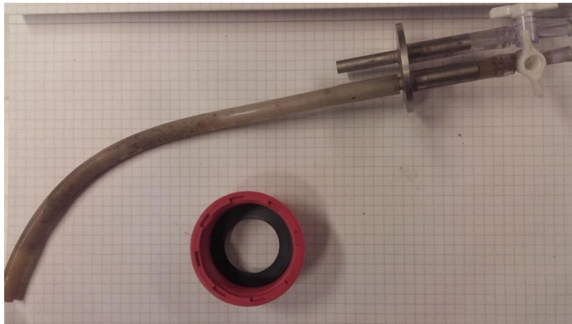
Figure 3-1 : Upper part : headpiece with its PVC tubes and two way valves. Lower part : hollow cap with the silicone seal inside. Used on top of the PR
