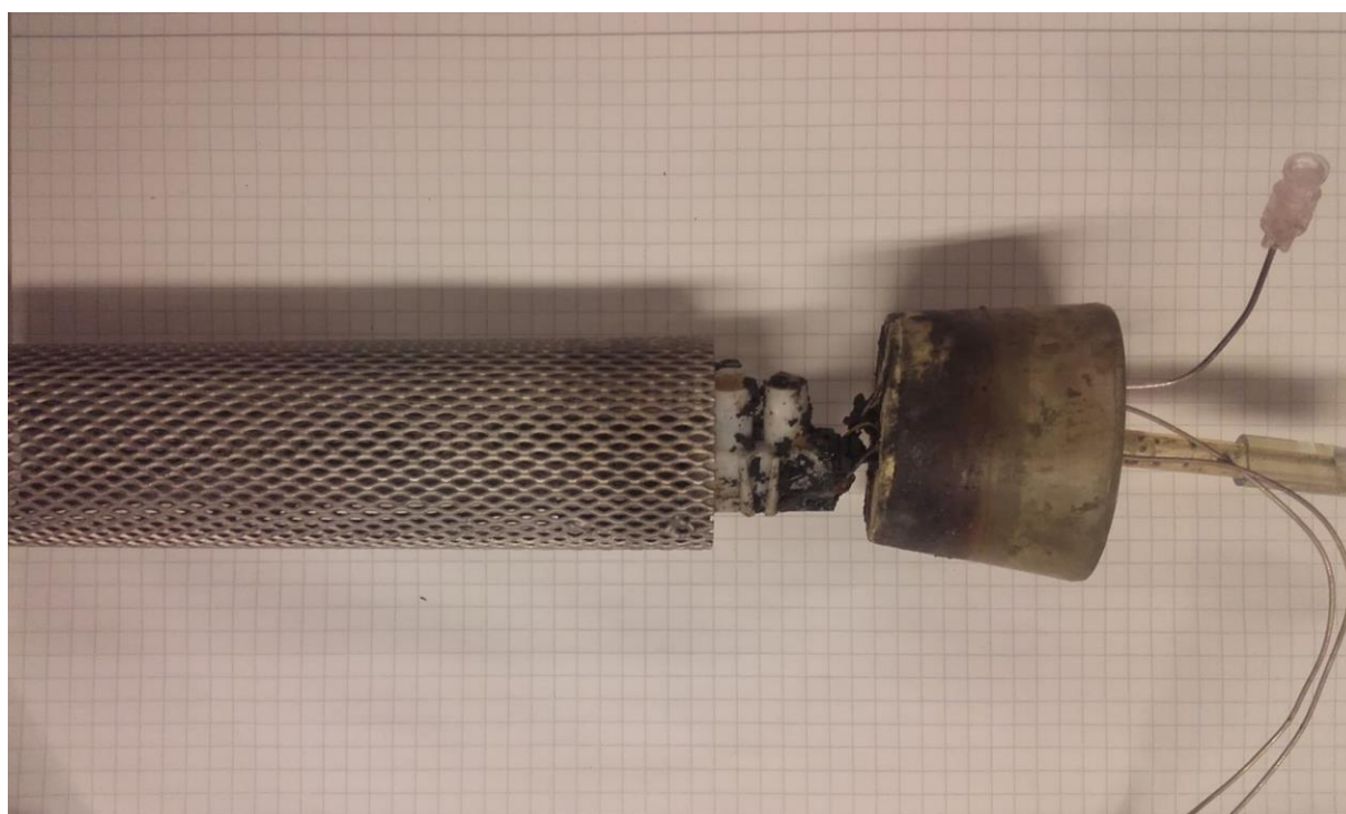
Figure 3-5 : anode connected to the silicone plug with the upper gas tube coming out at the upper side, the outflow tube in the middle and the connexion cable for the anode
