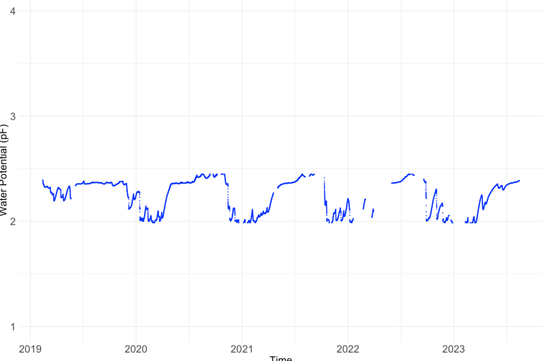
Evolution of Water potential over time for R10 at 2m with the raw data (Filtered data, hourly data)
