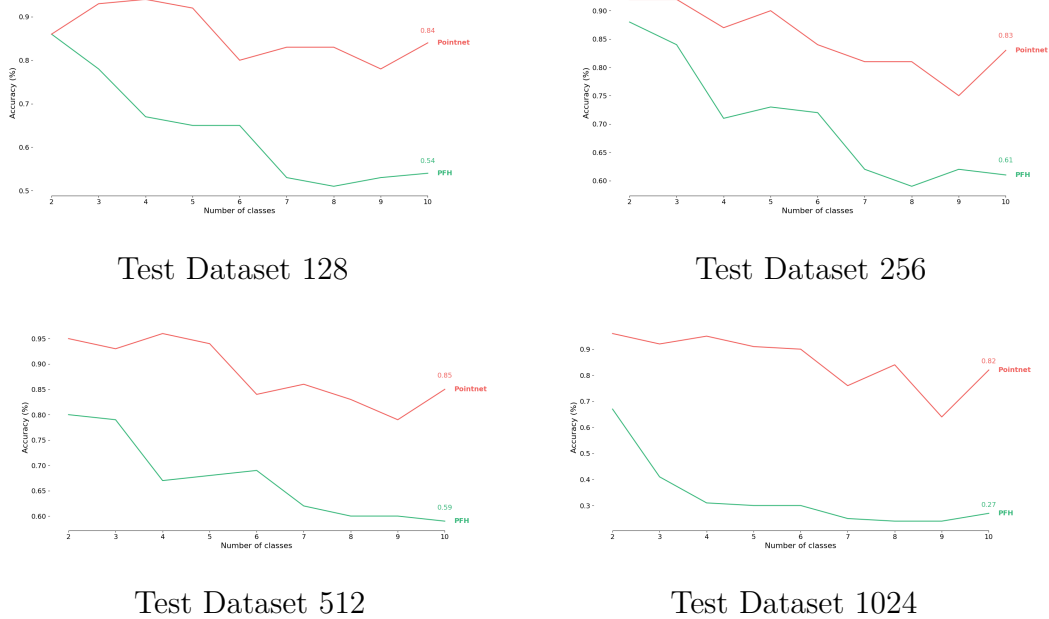
Figure 5.9: PointNet vs. Point Feature Histogram (PFH) accuracy with respect to number of sampled points
