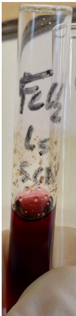
Picture 4. Fresh composition of \text{FeCl}_2 , \text{L}_5 and \text{SCN}^- , here are some orange crystals at top of the tube which look deliquescent
