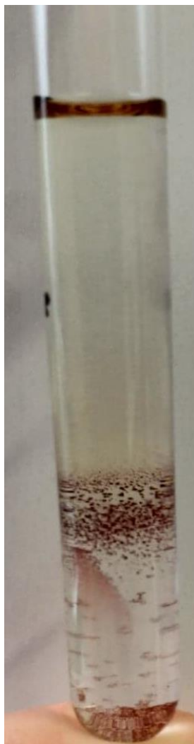
Picture 3. red crystals made of a composition of \text{Fe}(\text{BF}_4)_2 \cdot 6\text{H}_2\text{O} , \text{L}_5 and \text{SCN}^- . The ones made of a composition of \text{FeCl}_2 , \text{L}_5 and \text{SCN}^- look similar. When it is freshly made and before the collect, we can observe a sort of planar crystals but it disintegrates into smaller particles when collected.
