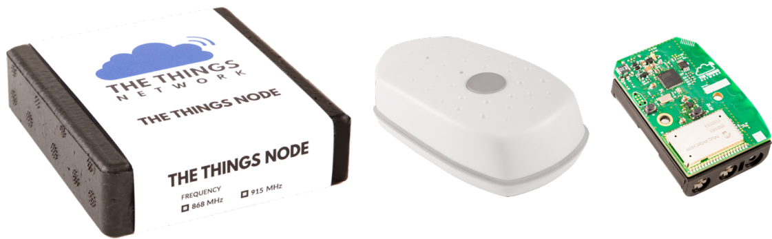
Figure 3.3: TTN node in its box and its casing, and the Printed circuit board
