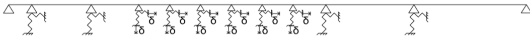
Figure 3.2.4 Correct static scheme of the footbridge accounting for tendons and their pretension.
