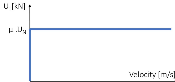
Figure 4.6 - Coulomb's friction model.
