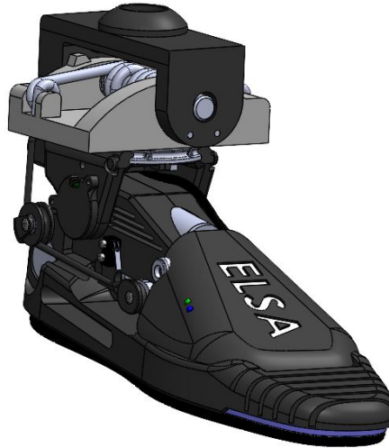
Figure 6.9: Global CAD view of the mechanism fixed on top of ELSA, an existing active prosthesis[37].
