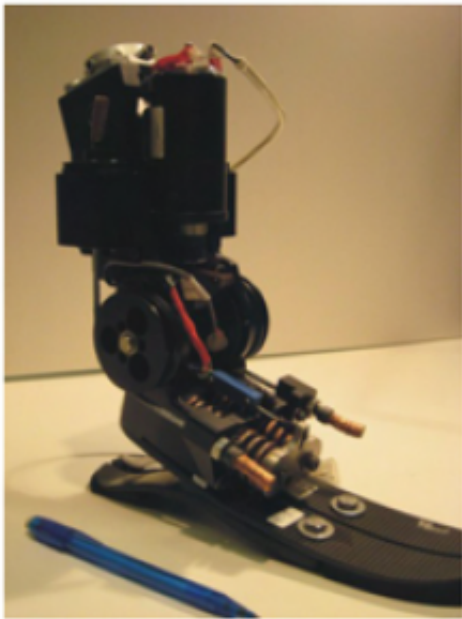
Figure 2.22: Physical prototype of the powered ankle-foot prosthesis developed by Herr et al. [28]
