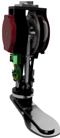
Figure 2.24: Powered ankle prosthesis developed at the Robotics Institute University of Michigan[31]
