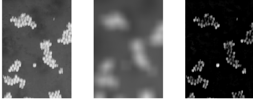
FIGURE 2.5 – (a) Originale - (b) Convolution Gaussienne - (c) Intensity high-pass
