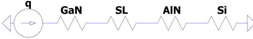
Figure 2.5: 1D thermal equivalent circuit for the model structure.
