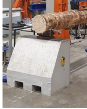
FIGURE 3.22 – Support en béton
