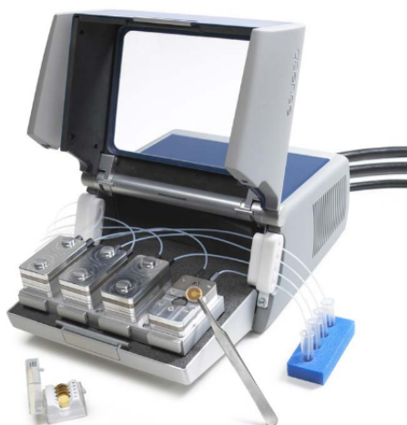
Fig. 34. Quartz crystal microbalance instrument, with four operating cells containing quartz crystals [47].
