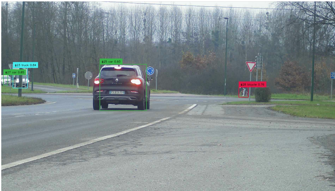
Figure 19: Example of output of YOLOv8. All the targets are detected. As expected, confidence level of smaller targets are smaller than for bigger targets
