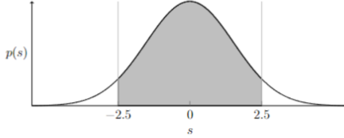
Figure 3.4: Gaussian density function of a scenario space of a single dimension. The shaded area encompasses 90% of the scenarios.
