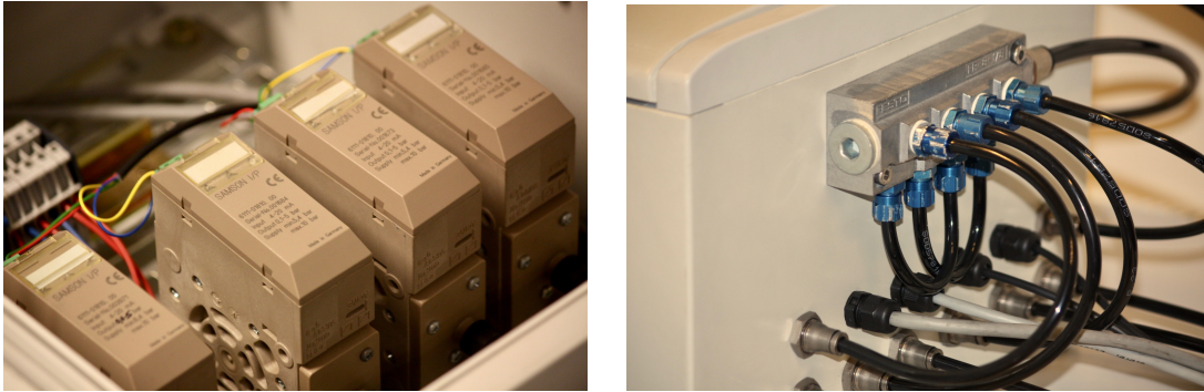
Figure 2.12: The Intensity/Pressure converters and the tubes.
