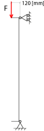
Figure 3.9: The load F is applied along y axis and the amplitude is 1 [kN/sec] (compression) given by loading function F1PS.
