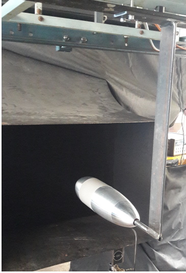
Figure 4.5: Zero degree angle of attack experiment
