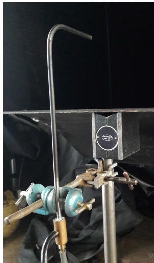
Figure 2.2: Pitot tube of the iMMC-LEFT wind tunnel
