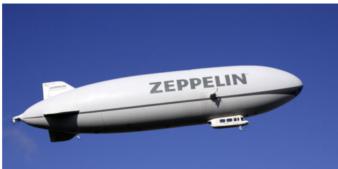
Figure 5: Zeppelin NT semi-rigid airship inflated with helium - 1997 [4]
