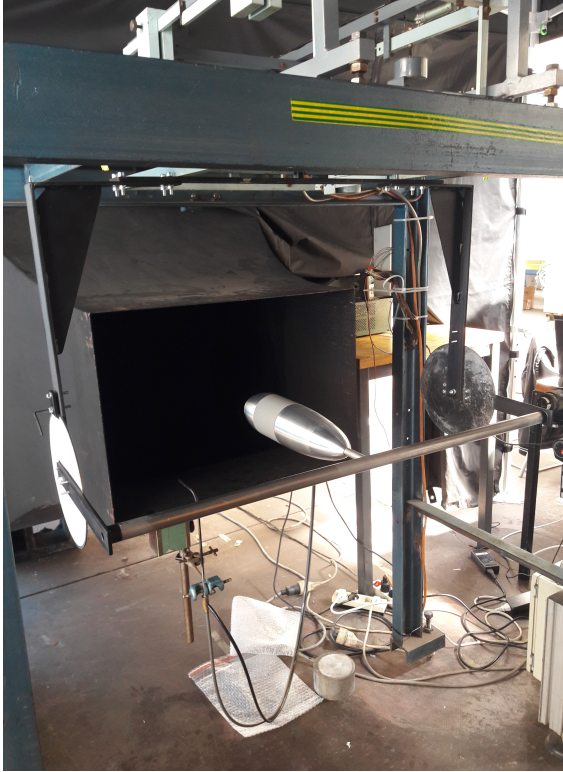
Figure 4.7: Smooth airship in wind tunnel (EXP1)
