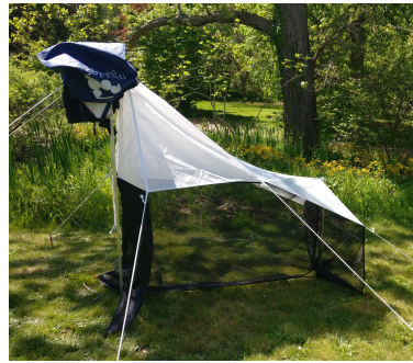
Figure D.2: Trap installed outside with cover on the monitoring box
