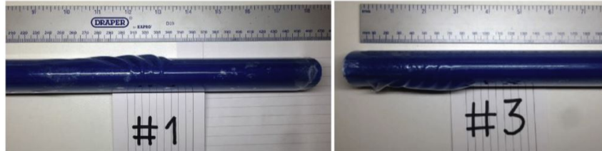
Figure 3.7: Significant tape detachment and water entrapment in sample 1 after 8h and in sample 3 after 5h of rain erosion testing. Reprinted from [4]
