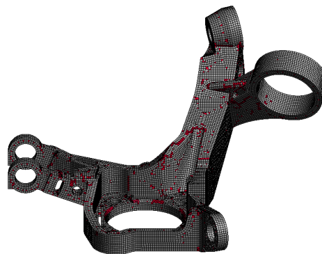
(f) Output mesh generated for Fusee_1 (quality threshold: 0.1). This mesh contains 49,563 hexahedra and 48,253 tetrahedra. The worst hexahedra has a quality of 0.101.
