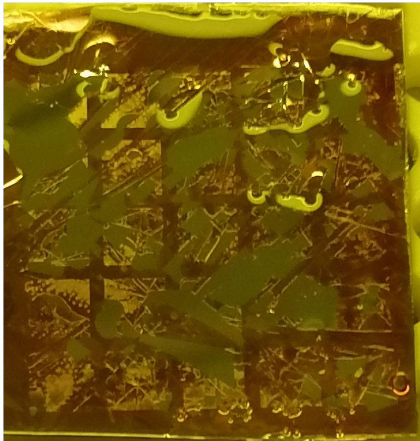
Figure A.0.12: Illustration of stripping marks due to the overdevelopment of AZ9260 . The sample was placed for 30 minutes in AZ700MIF , a developer.
