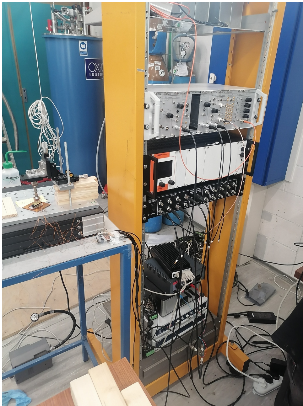
Figure A.0.21: Homebuilt AFM set-up, the piezotube, piezomotor, tuning fork and sample are placed on a damping table. A close-up view of these elements is provided at Figure A.0.22. The control units are connected to a computer not shown.
