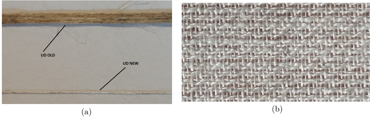
Figure 4.1: Used flax reinforcements for this work (a) strand structure for both UD reinforcements: "UD OLD" strand is an assembly of non-twisted fibers while "UD NEW" strand is a twisted yarn (b) flax twill fabric structure. The strands are twisted yarns as well.
