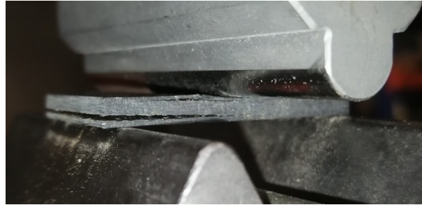
Figure 6.4: Typical delamination defects found on carbon samples after water cutting. Remark: the sample is not loaded.
