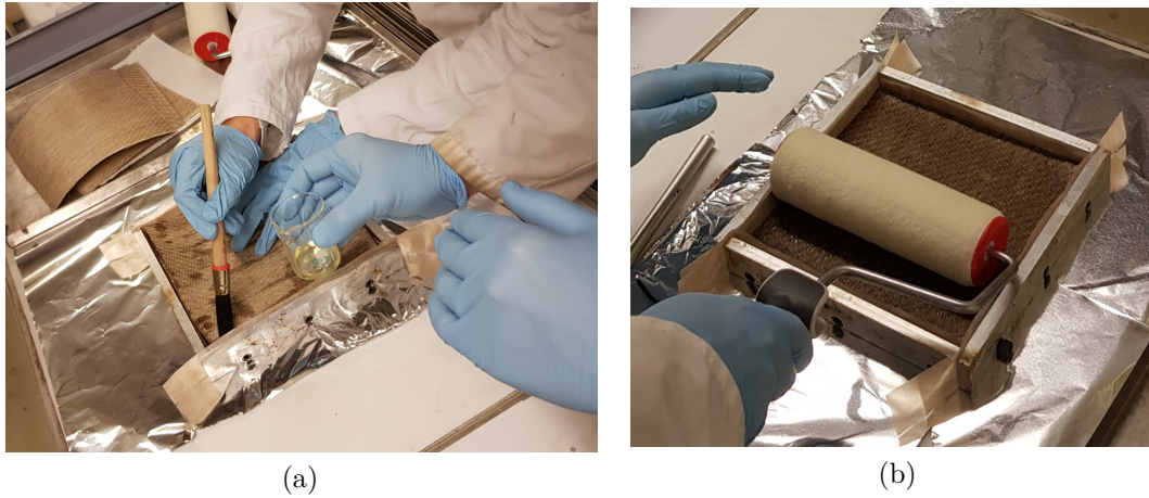
Figure 4.2: Impregnation of small laminates using the hand layup technique.
