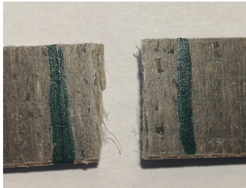
Figure 5.5: Tensile specimen failure after the tensile test in the transverse direction.
