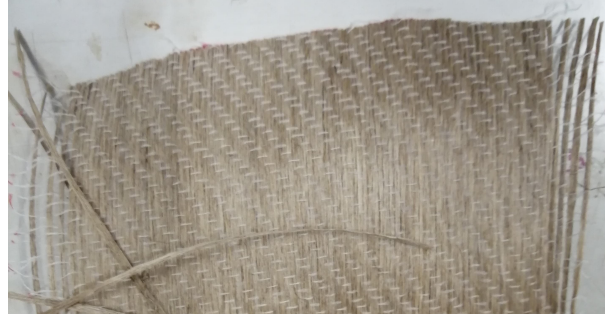
Figure 6.1: Delamination of the fibers during the cutting of the first plies.
