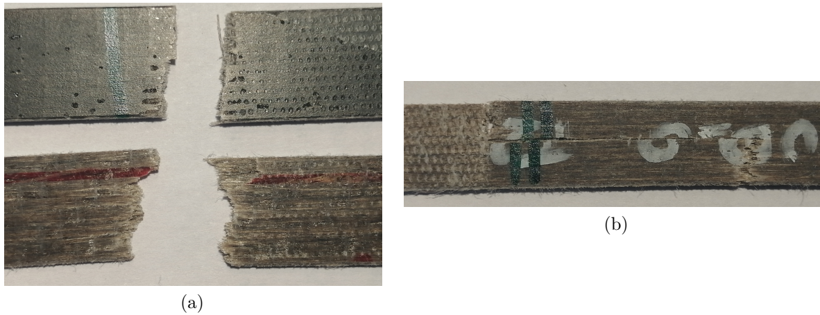
Figure 5.2: Tensile specimens after failure in the fiber direction (a) specimens with a failure perpendicular to fibers. On the top, specimens was manufactured with the new UD fabric and on the bottom, the specimen was manufactured with the old one (b) Two cracks perpendicular to fibers located at the two extremities of the sample joined by a longitudinal one.
