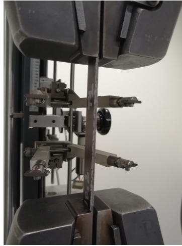
Figure 4.7: Installation for tensile test. The sample is maintained by the grips and each extensometer arm is touching sample surface at one point during loading.
