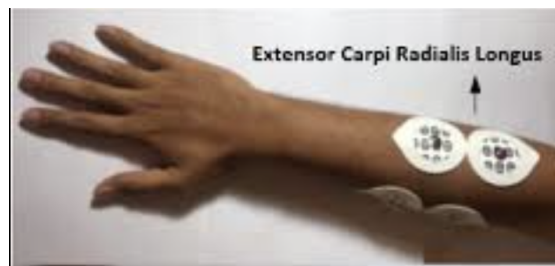
Figure 2.2: Illustration of the placement of the electrodes on the wrist extension muscles (missing the ground terminal) [15].
