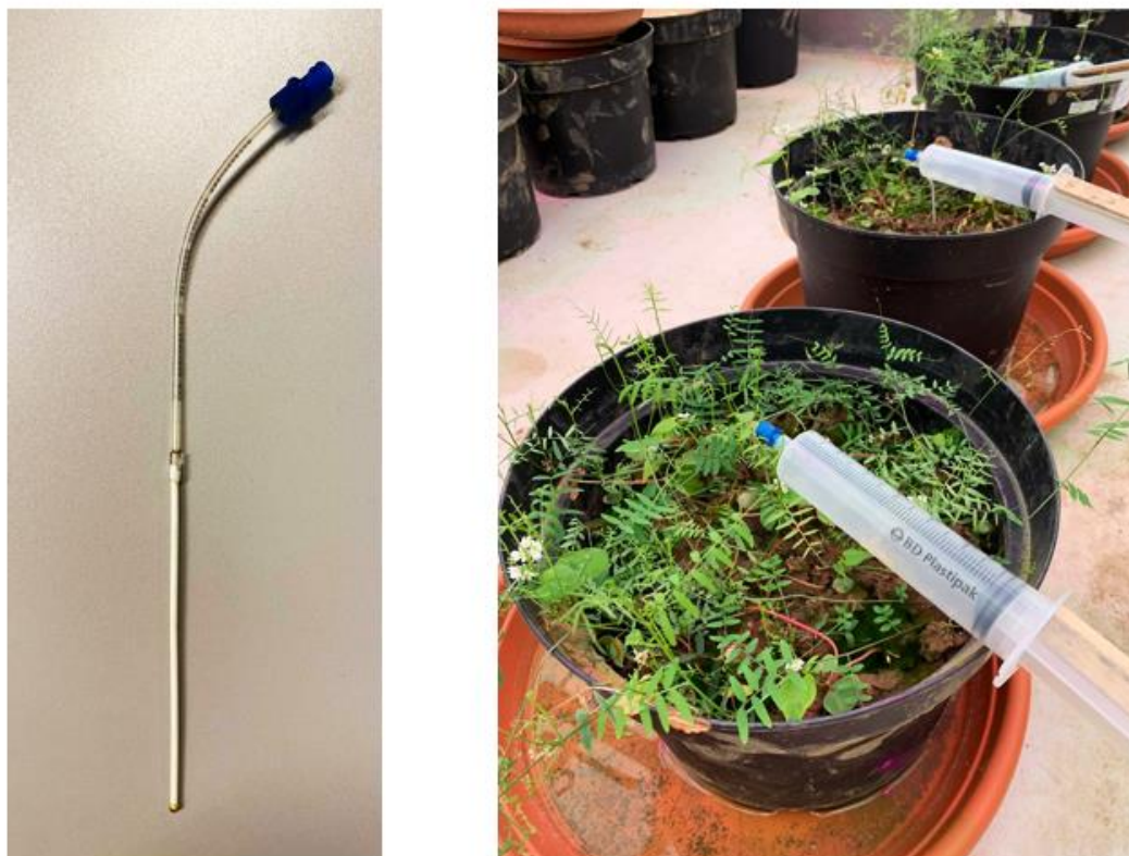
Figure 4-6: Micro-rhizon (A). Syringe connected to a micro-rhizon to collect a pot soil solution (B).
