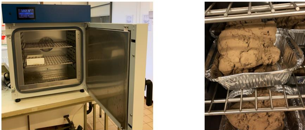
Figure 4-5: Oven in the MOCA laboratories (ELI, UCLouvain; A ). Dried soil sample after 24 hours in the oven ( B ).
