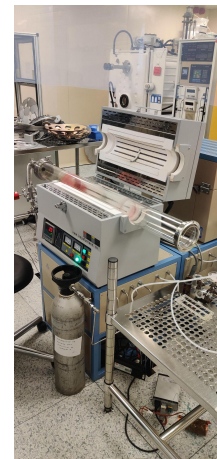
Figure 4.7: Photo of our furnace in Winfab cleanroom, the horizontal tubular chamber
