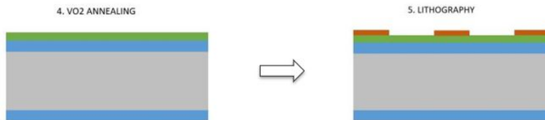
Figure 4.12: Cross section of the photolithography microfabrication step [37]. The color gray represents Si, while blue represents SiO 2 , green is crystallized VO 2 and orange the photoresist.
