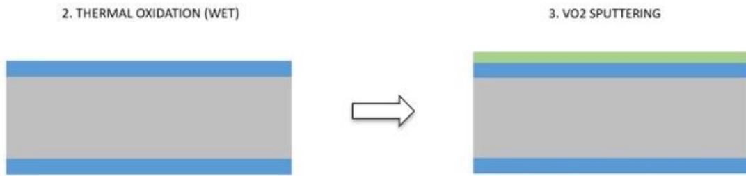
Figure 4.6: Cross section of the sputtering microfabrication step [37]. The color gray represents Si, while blue represents SiO 2 and green VO 2 .
