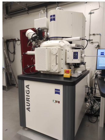
Figure 5.1: EISS focused ion beam scanning electron microscope (SEM) used in the Winfab lab
