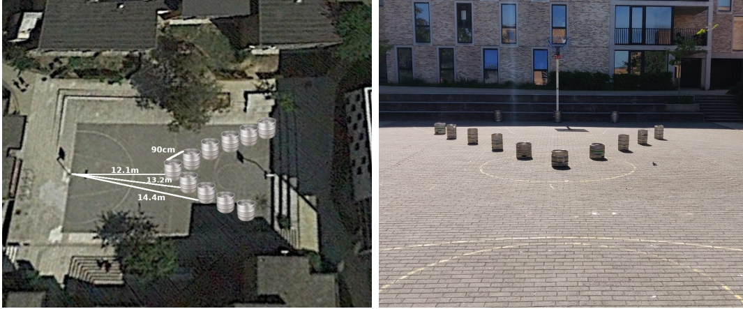
Figure 7.16: Satellite view (left) and radar view (right) of the setup of the measurements performed to quantify the impact of setup imprecision. Ten barrels had been placed in a triangle shape at a distance L_{\text{target},0} = 12.1 [m] . Distance between barrels is 90 [cm] . The tilt angle of the radar was 0^\circ and its height 90 [cm] .
