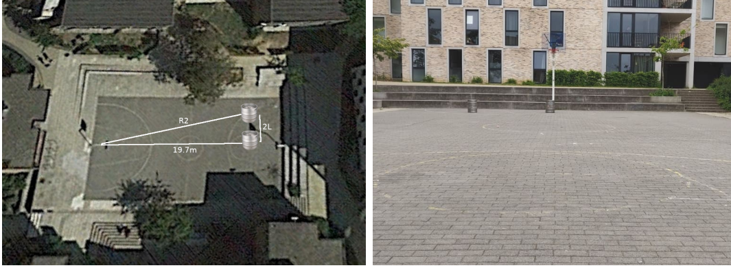
Figure 7.10: Satellite view (left) and radar view (right) of the setup of the measurement performed with two barrels. The radar is placed at 19.7 [m] from the first barrel. The distance between barrels will vary between 2L = [10 \ 4 \ 3 \ 2 \ 1 \ 0.5 \ 0.2] [m] . R_2 can be computed for each value of 2L . The tilt angle of the radar with regards to the horizontal was 0^\circ and the height of the radar compared to the ground was 90 [cm] .
