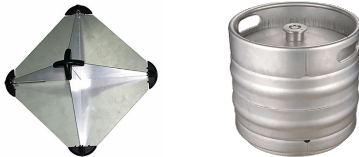
Figure 7.1: Target (left) and barrel (right) used as reference for the measurements. The target measures 45.72 [cm] at its diagonal. The dimensions of the barrel are (Height, Diameter) = (53.2, 40.8) [cm] .
