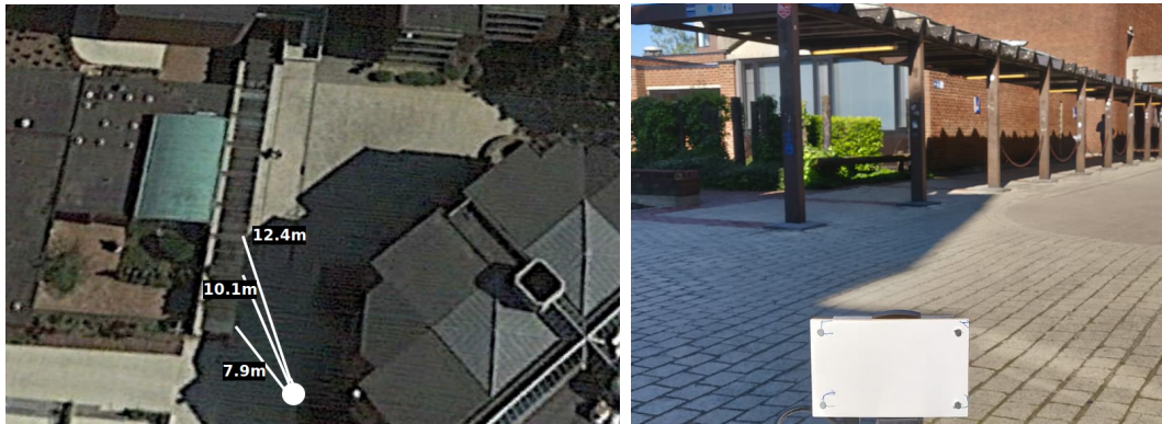
Figure 7.7: Satellite view (left) and radar view (right) of the setup of the Barbe entrance measurement. The radar is placed at 7.9 [m], 10.1 [m] and 12.4 [m] of the first three poles. The tilt angle of the radar with regards to the horizontal was 0^\circ and the height of the radar compared to the ground was 90 [cm]. A pole measures 20 \times 12 [cm].
