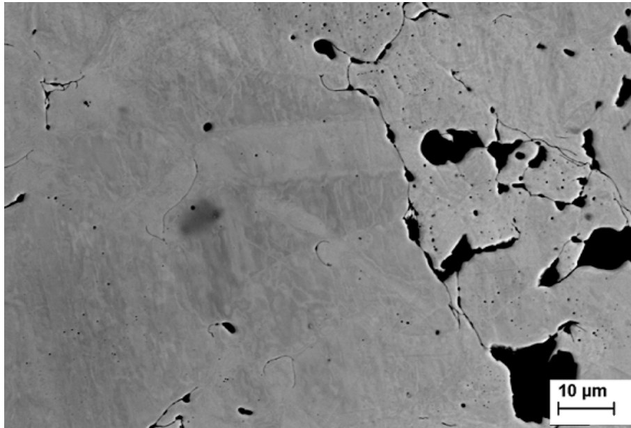
Figure 3.3.3: SEM Image showing the presence of twins in FeMnCoNiZn alloy after heat treatment - Case 1B
