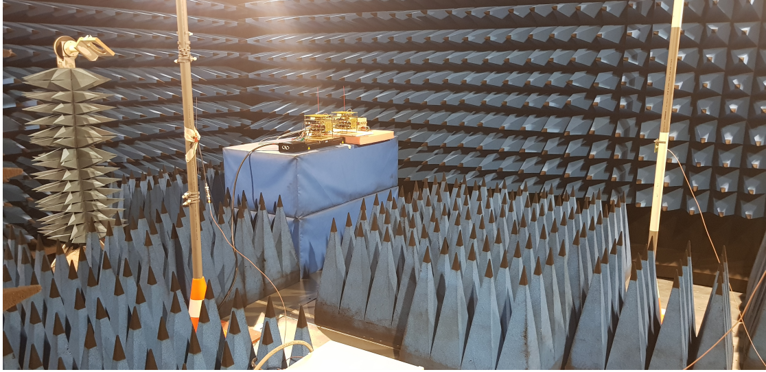
Figure 22: Setup anechoic chamber
