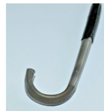
Figure 4.4: Tube bended in the right shape with a 3D-printed bender but obstructed with melted sand.
