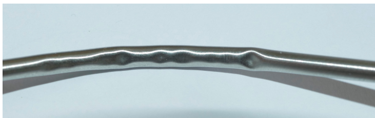
Figure 4.3: Bending failure with wrinkling.
