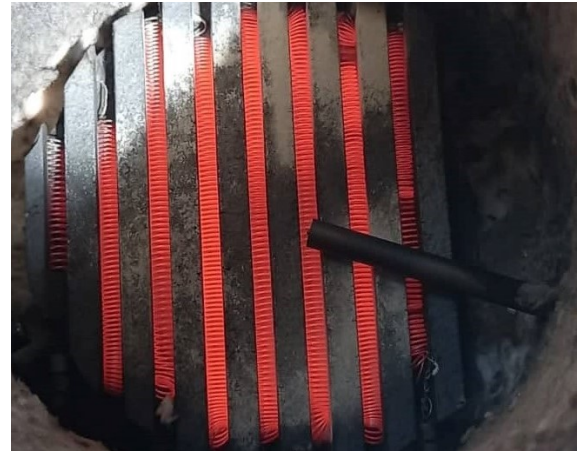
Figure 4.2: Protecting ceramic tube above the wire
