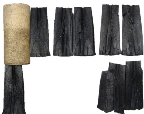
Figure 4.8: Radial and axial shrinking
