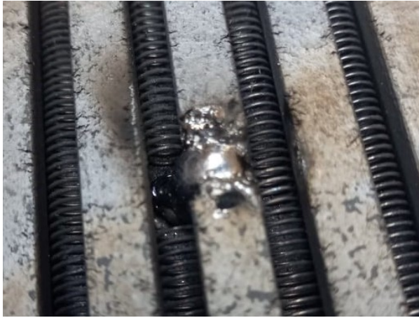
Figure 4.1: Melting of the probe on the ceramic
