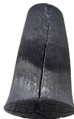
Figure 4.9: Sample splitting side view
