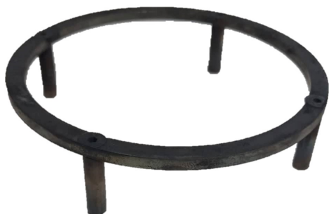
Figure 3.5: Metal base of the heating ceramic
