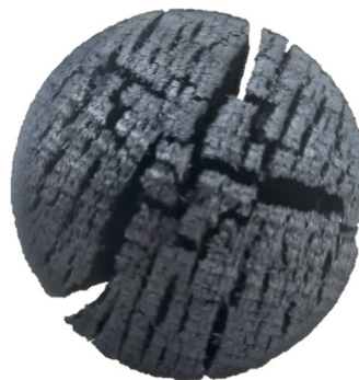
Figure 4.11: Sample splitting bottom view
