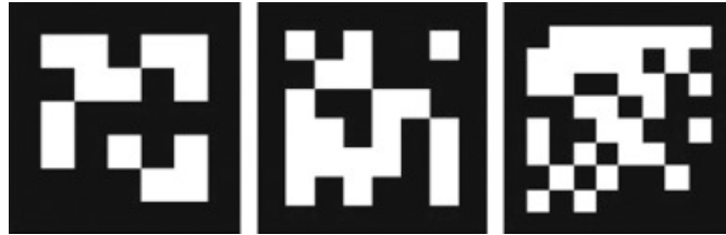
Figure 4.9: ArUco square markers used for detection, with a resolution of 5x5, 6x6 and 8x8 respectively[22]
