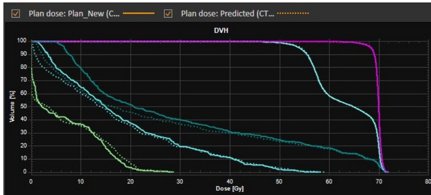
Figure 5.7: DVH curves of the prediction in dotted line and of the conventional plan generated in solid line. The pink curve represents the CTV boost of 70Gy, the light blue is the CTV prescription of 54.25Gy and the others are the spinal cord and parotids.
